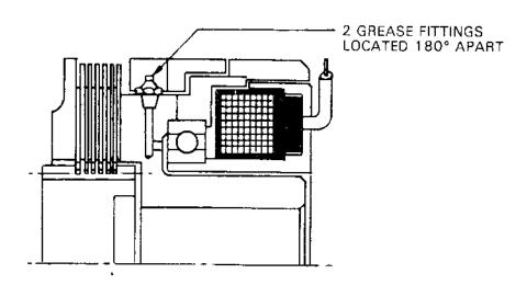
The clutch should be lubricated after about every 200 hours of operation. The interval between lubrication can be increased or decreased depending upon the severity of the application. Both fittings should be greased until the grease starts to come out of the relief slots—AVOID OVER-GREASING.
